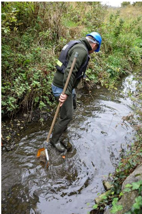
Plate 7.6 Q-sampling the Cuckoo stream (site 6), also grossly polluted and unsuitable for fish life
